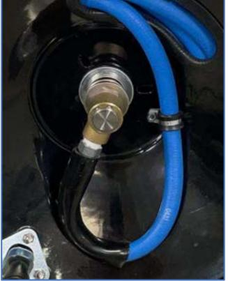
Picture to the left: Install rubber coated clamp around the hose. Use self-tapping screw to tighten clamp onto hose reel.
